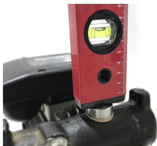
Figure 14. Leveling it in the X direction
