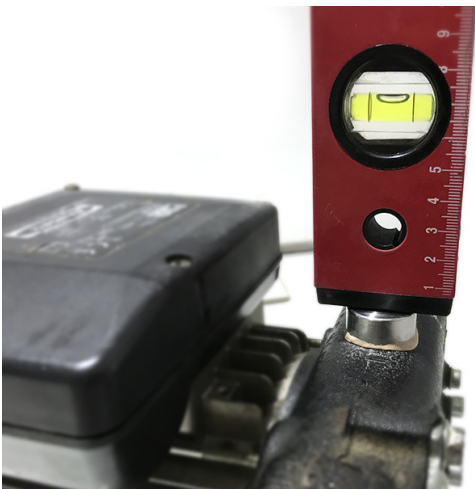
Figure 15. Leveling it in the Y direction
