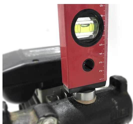
Figure 14. Leveling it in the X direction
