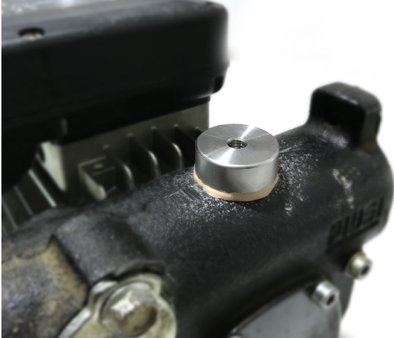
Figure 13. Place the base with Epoxy on the equipment's surface
