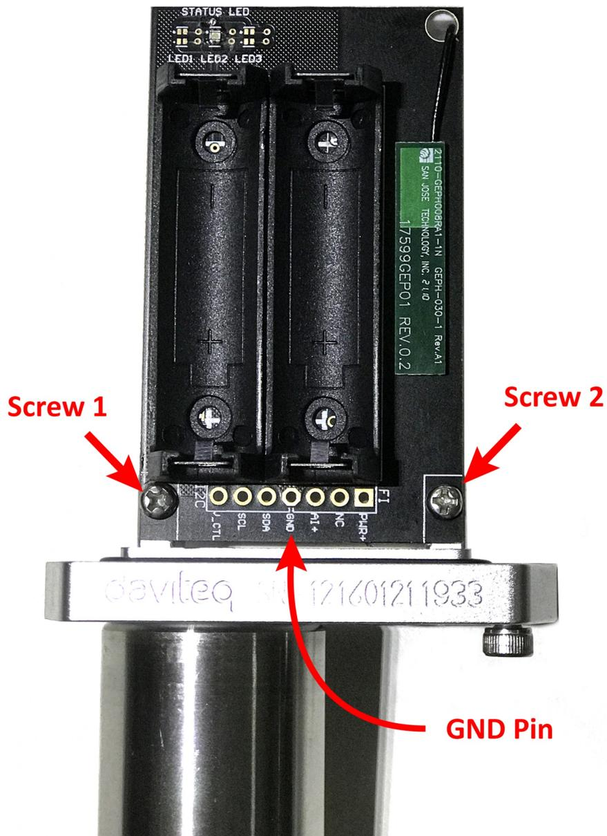
**Step 3:** Solder a wire to this GND point; the other end of the wire will be screwed to 1 of 2 screws on the aluminum base;
