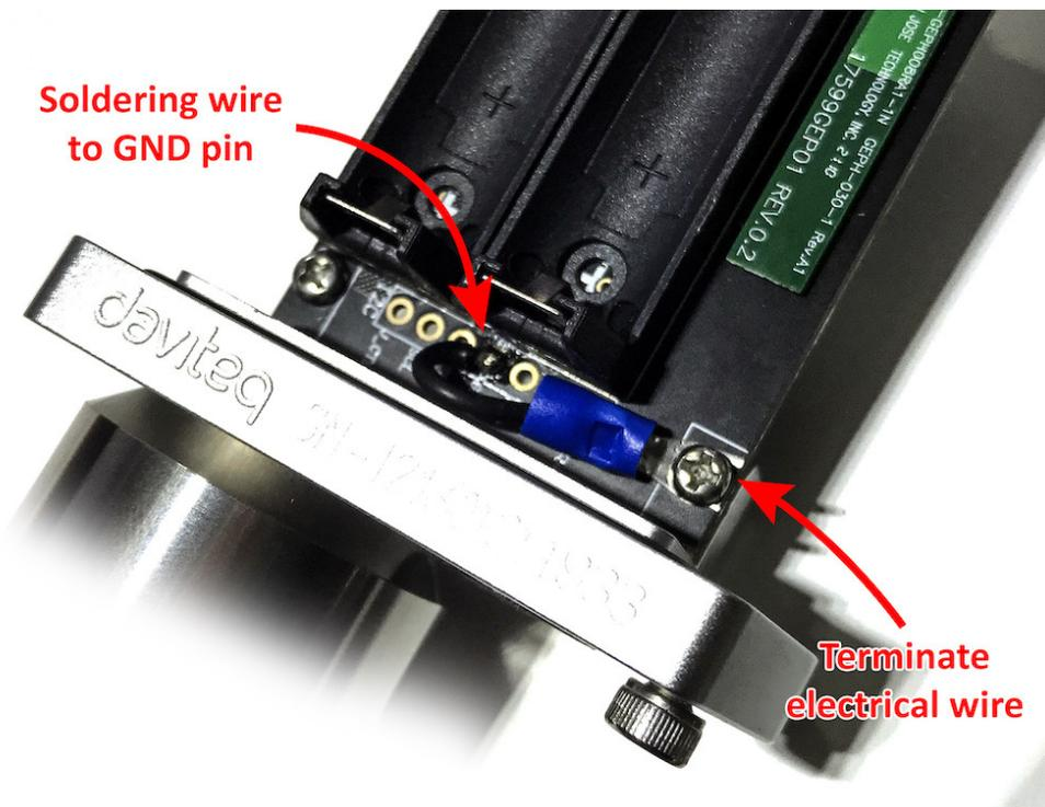
**Step 4:** Outside of the aluminum base there is another screw → make a wire connection from this screw to the body of pressure sensor (stainless steel cylindrical body) → Use a hose clamp or stainless steel pipe bracket to lock the connection between the wire and the housing.
