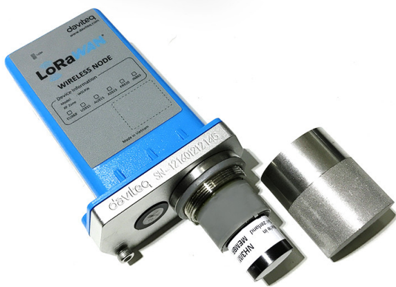
Step 1. Remove the filter
