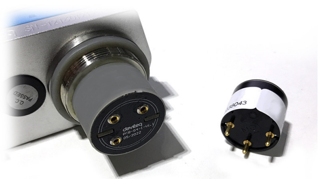
Step 2. Unplug the sensor module
