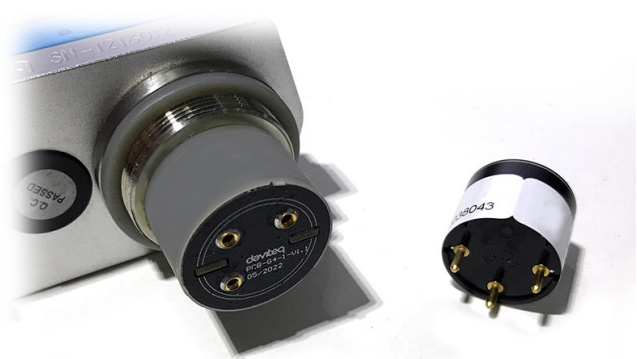
Step 2. Unplug the sensor module
