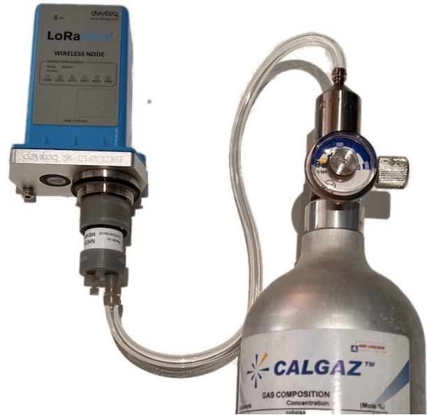
Step 4. Attach the tube to the regulator
