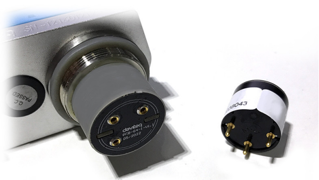
Step 2. Unplug the sensor module
