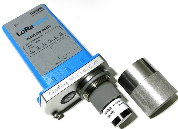
Step 1. Remove the filter
