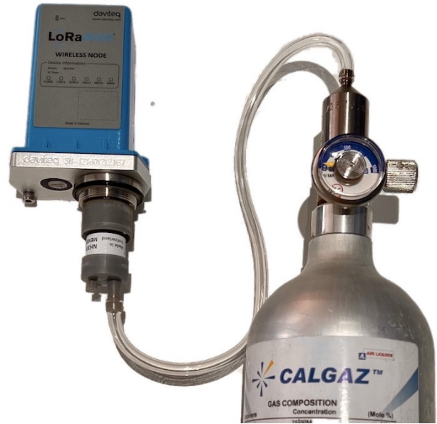
Step 4. Attach the tube to the regulator
