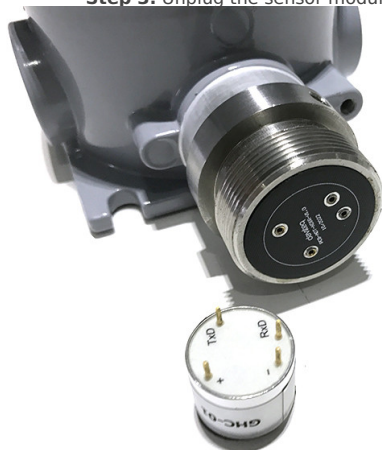
Step 3. Unplug the sensor module
