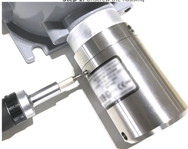
Step 1. Unscrew the housing
