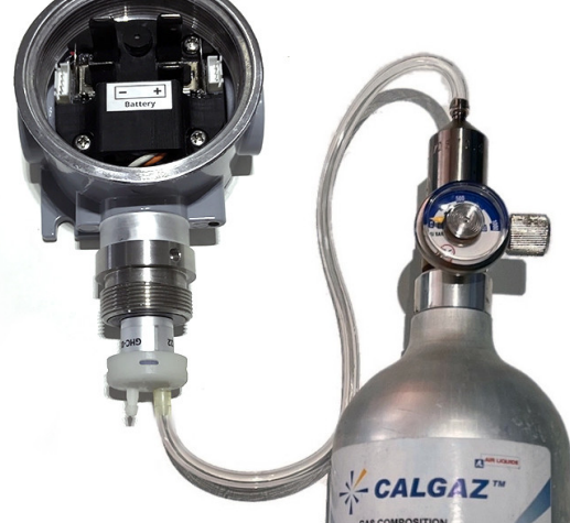
Step 4. Attach the tube to the regulator
