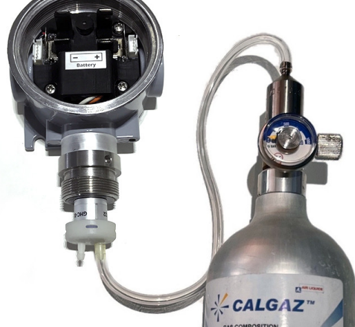
Step 4. Attach the tube to the regulator
