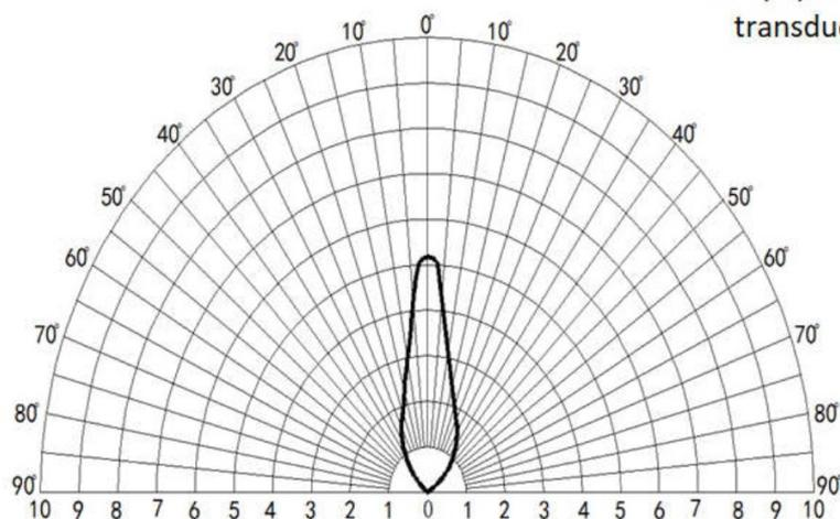
Cambered surface beam pattern of paper sheet Unit: meter
