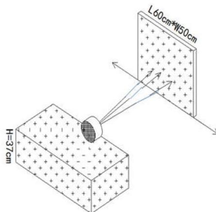
The smart firmware allows the sensor to filter the wrong echo signal from a rough surface in the trashbin so that it can deliver the accurate average distance or level value.
