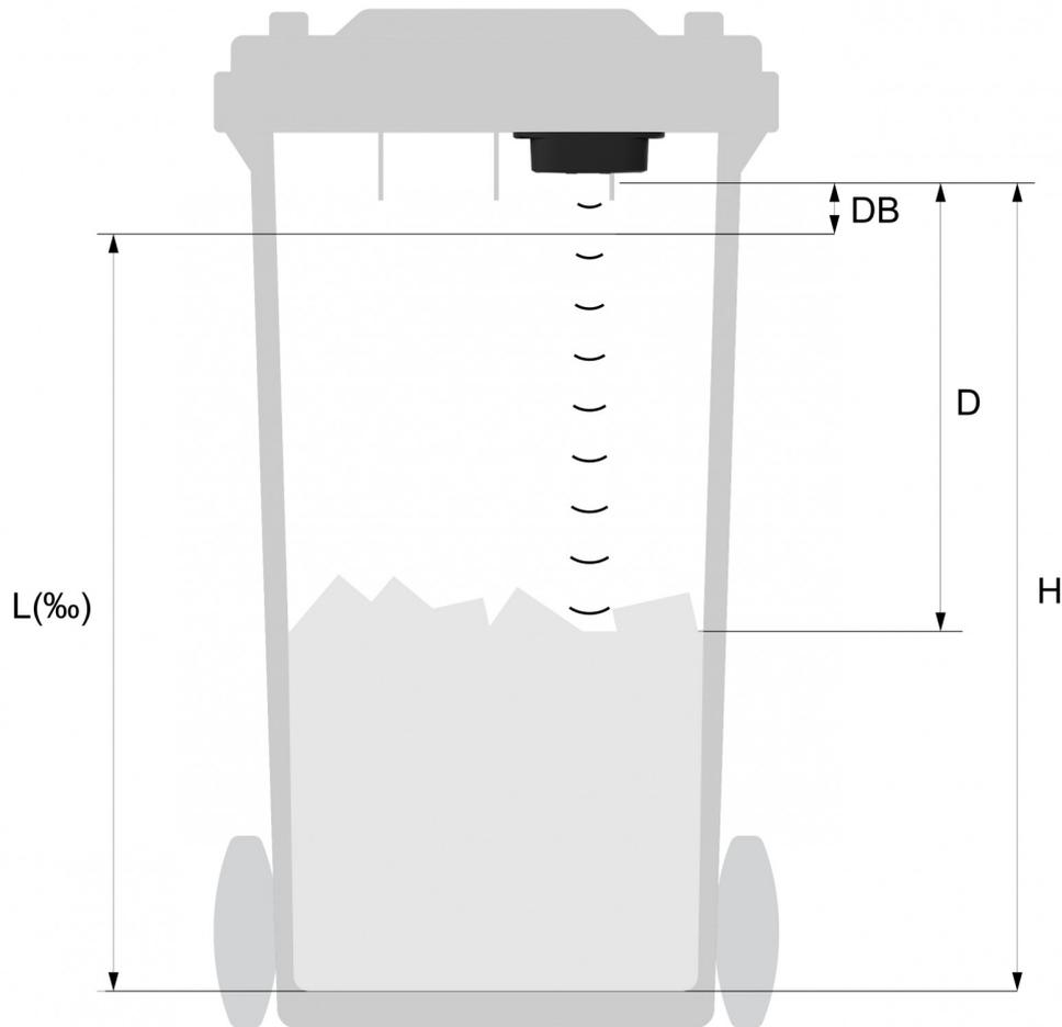
**DB:** Dead band = 30 mm (This is a short range in front of the ultrasonic sensor can't measure distances)
