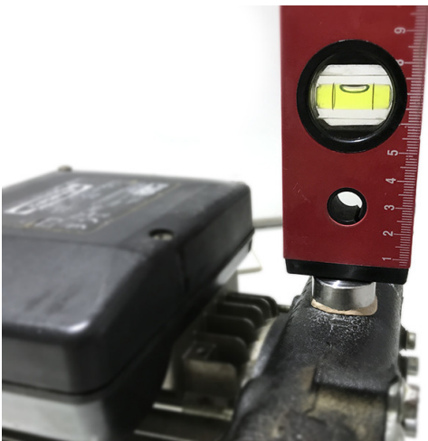
Figure 15. Leveling it in the Y direction
