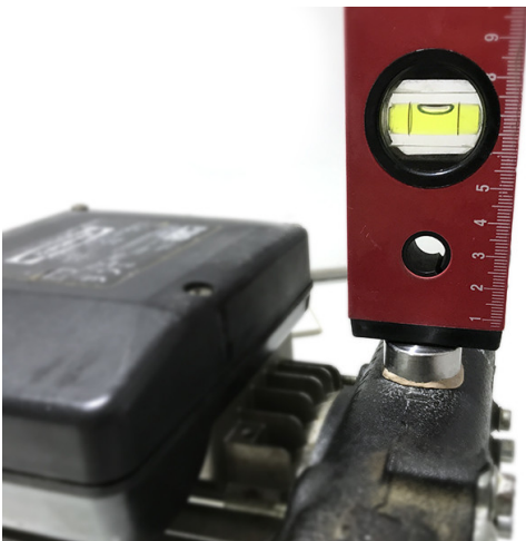
Figure 15. Leveling it in the Y direction
