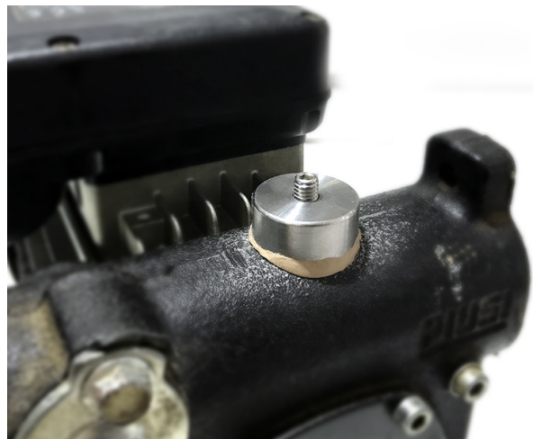
Figure 16. Leave it dry for 24 hours before installing the sensor
