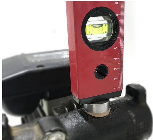
Figure 14. Leveling it in the X direction
