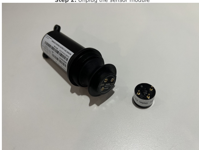
Step 2. Unplug the sensor module
