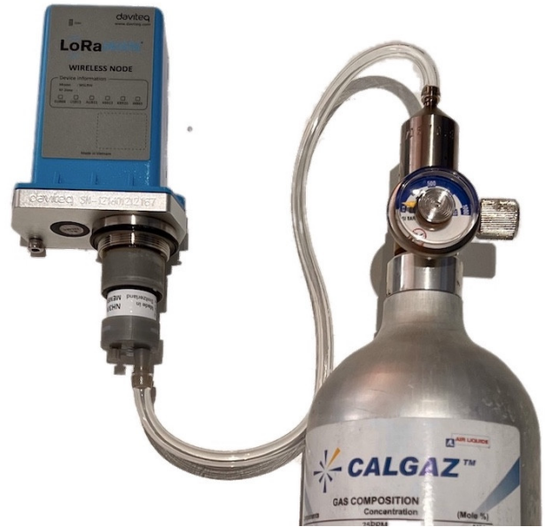
Step 4. Attach the tube to the regulator
