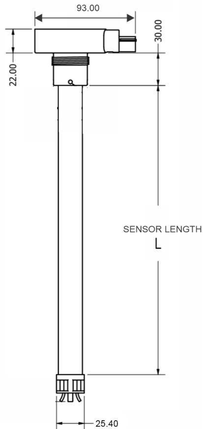
Sensor length is  $L = 2000$ ,  $H = 1700$  mm  $\Rightarrow C = 326$  mm  $\Rightarrow$  Cut the sensor pipe length of 326 mm.
