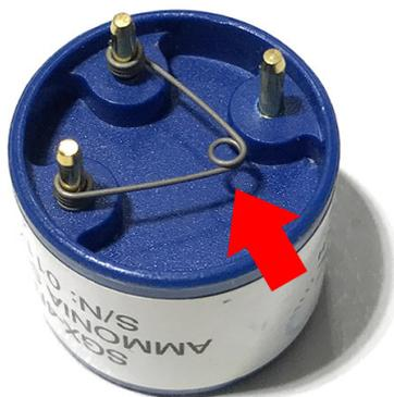
**Step 4. Plug the new sensor module into the PCB**
