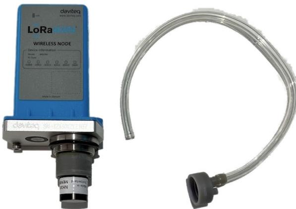
**Step 2.** Attach the calibration cap to the sensor head
