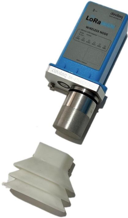
**Step 2.** Insert the rain guard into the sensor filter and tighten the locking screws
