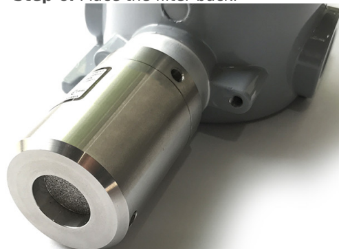
Step 6. Place the filter back.
