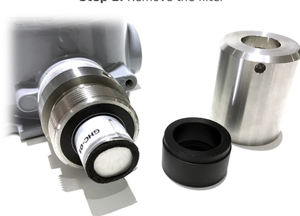
Step 2. Remove the filter
