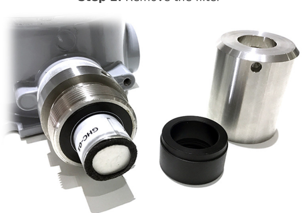
Step 2. Remove the filter
