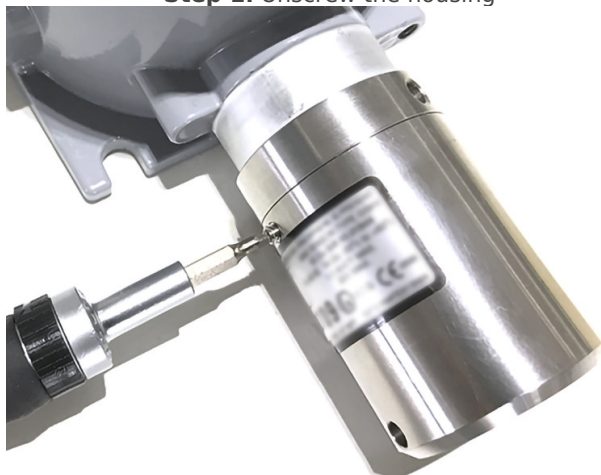
Step 1. Unscrew the housing
