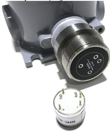
Step 3. Unplug the sensor module
