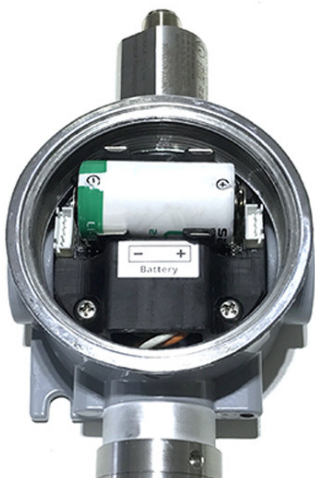
Step 5. Insert the batteries and start calibrating the new sensor as per section 3 .
