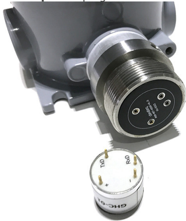
Step 3. Unplug the sensor module
