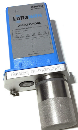
Step 6. Place the filter back.
