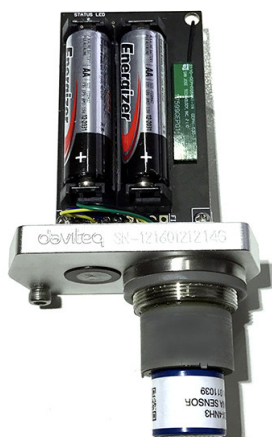
Step 5. Insert the batteries and start calibration of the new sensor as per section 3 .
