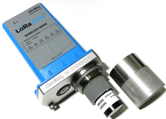
Step 1. Remove the filter
