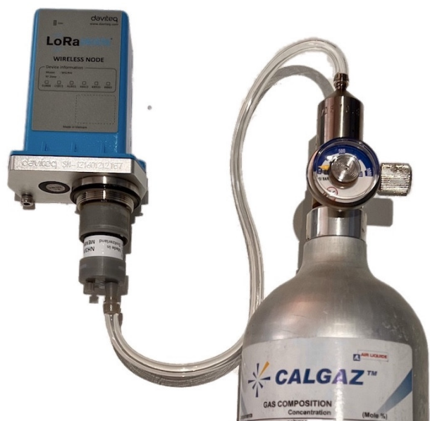
Step 4. Attach the tube to the regulator
