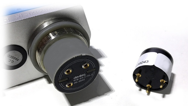
Step 2. Unplug the sensor module
