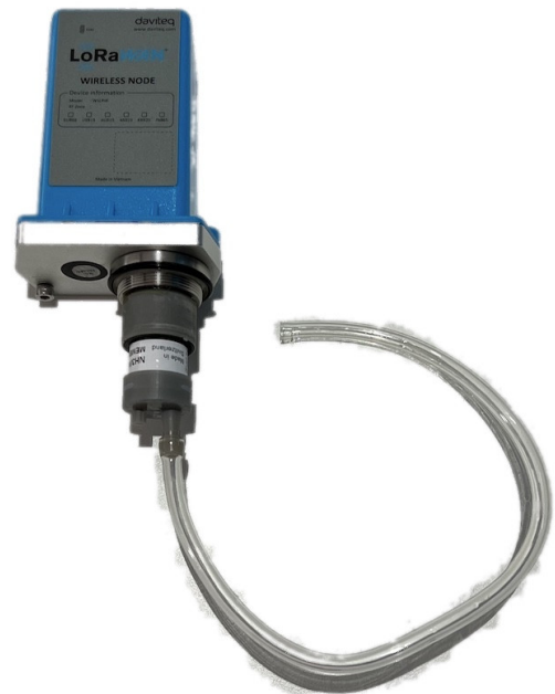
Step 4. Attach the tube to the regulator
