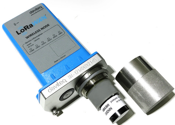
Step 1. Remove the filter
