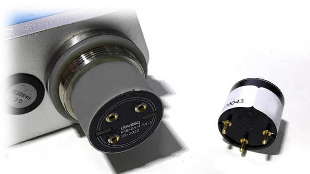
Step 2. Unplug the sensor module
