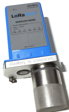
Step 6. Place the filter back.
