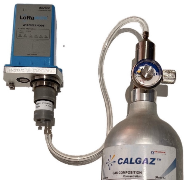
Step 4. Attach the tube to the regulator
