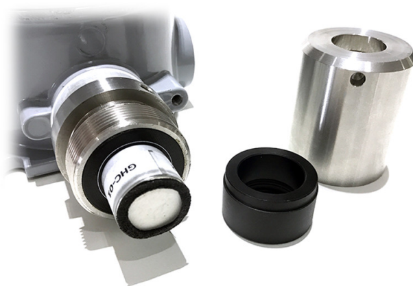
Step 2. Remove the filter
