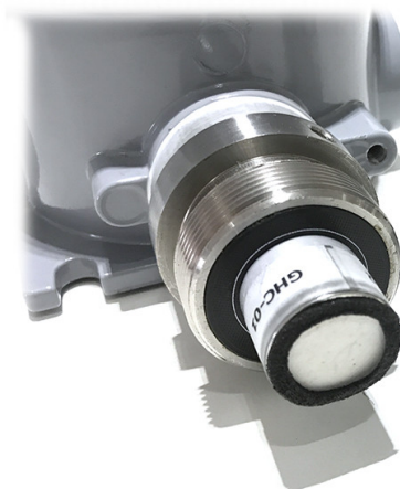
Step 4. Plug the new sensor module into the PCB
