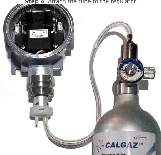
Step 4. Attach the tube to the regulator
