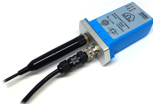
After powering iConnector Wifi, the led of Status and Network will blink alternately. That means iConnector Wifi is in access point mode.
