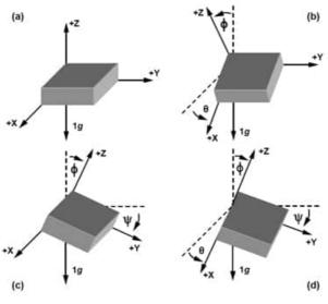
The AG Tilt sensor module measures the Acceleration of the 3-axis.
