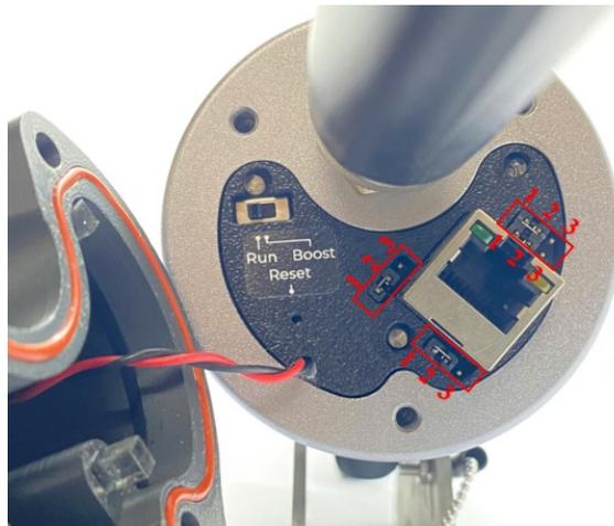
Only change the jumper position when **the gateway doesn't support PoE+ source 802.3at** but you want to power the gateway through ethernet cable as the below diagram.
