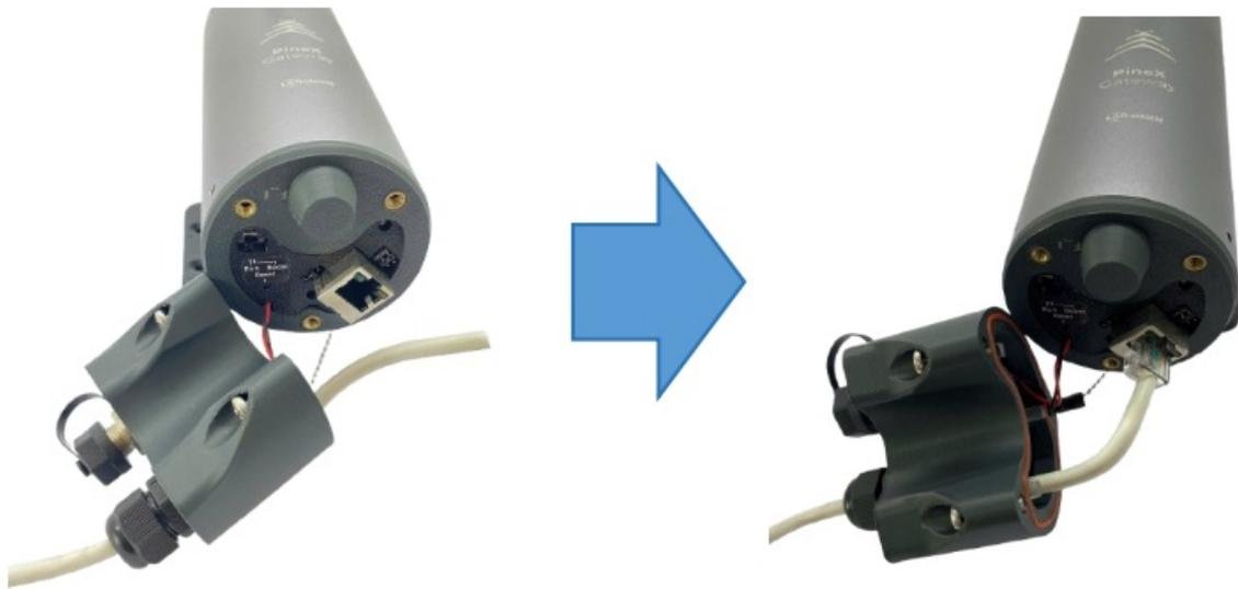
Step 4 : Close the gateway's cover, then use the screw driver to lock the 3 screws.
