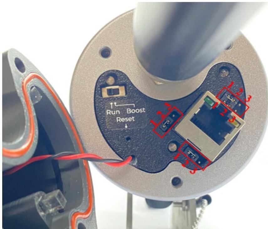
**1** Only change the jumper position when **the gateway doesn't support PoE+ source 802.3at** but you want to power the gateway through ethernet cable as the below diagram.
