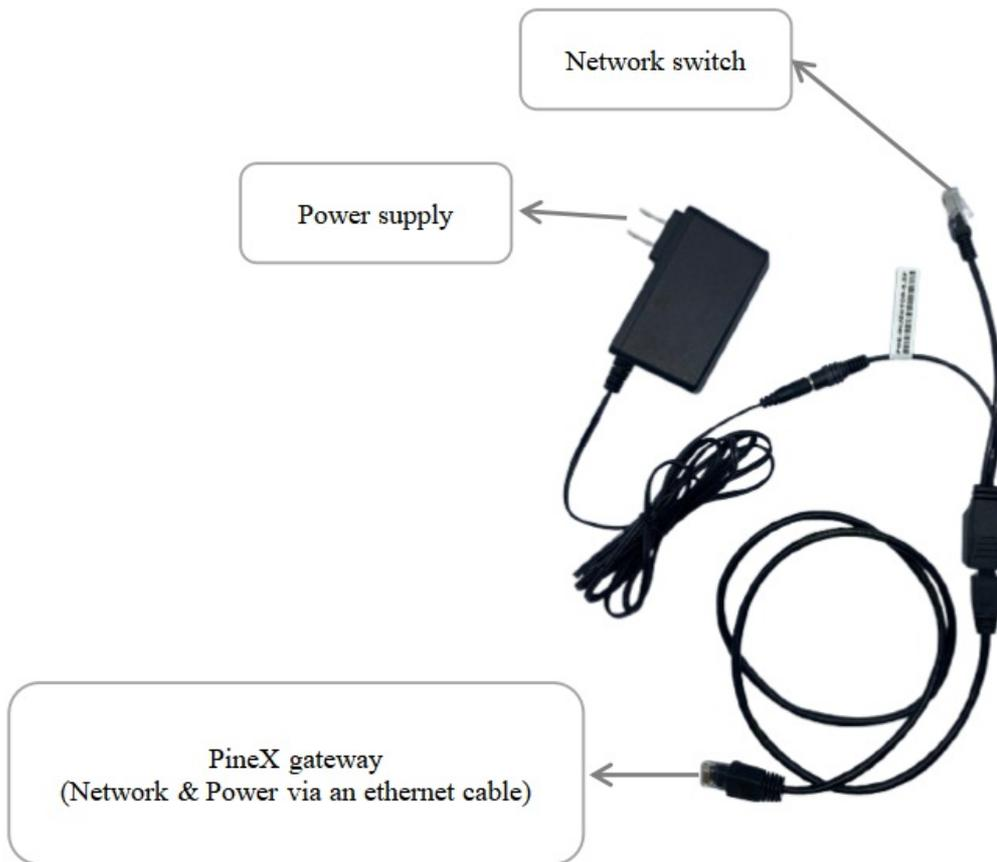
❗ To power the gateway through Ethernet cable as the above diagram, four jumpers have to change to connecting port 2 and port 3 as below
