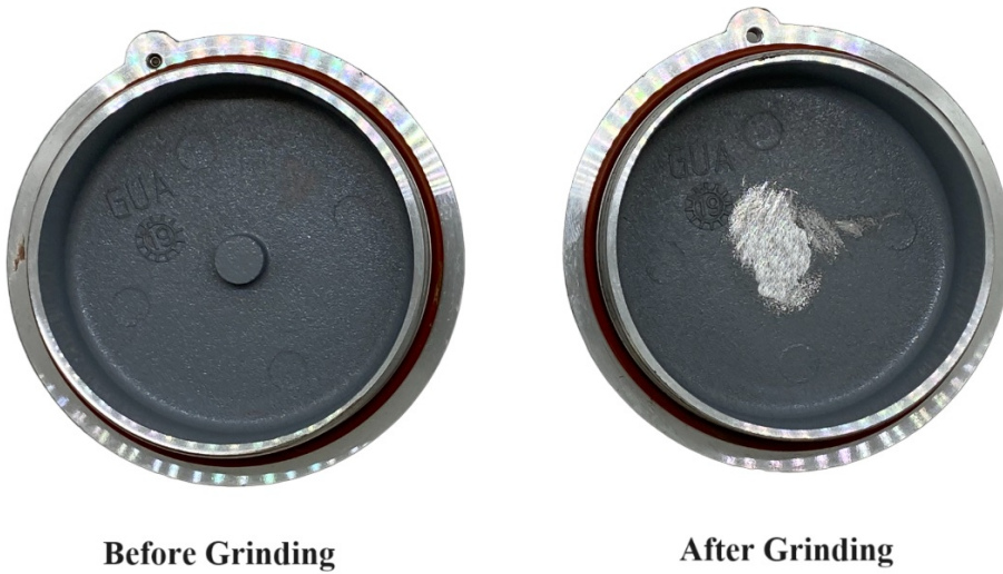
Figure 2.2: Grind the excess part inside the housing cover.
