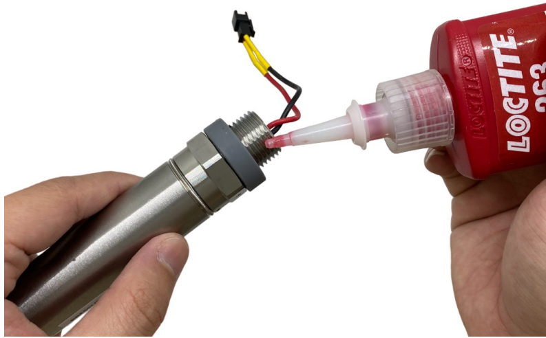
Figure 3.1: Apply thread lock glue to the connection thread of sensor.
