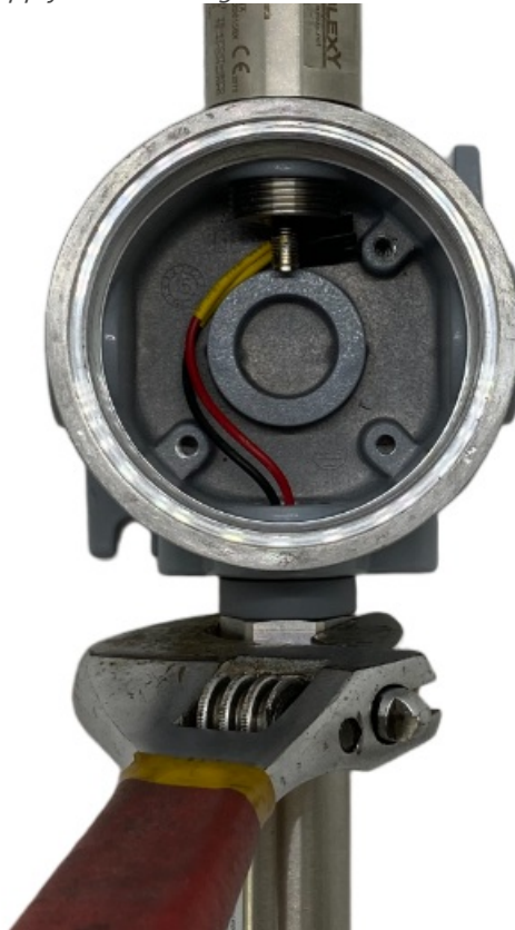
Figure 3.1: Apply thread lock glue to the connection thread of sensor.
