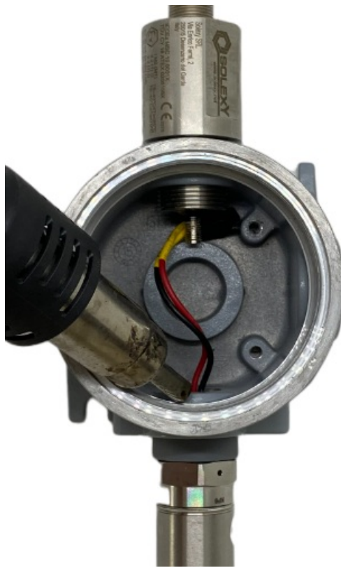
Figure 2.5: Heat up the connecting thread.
