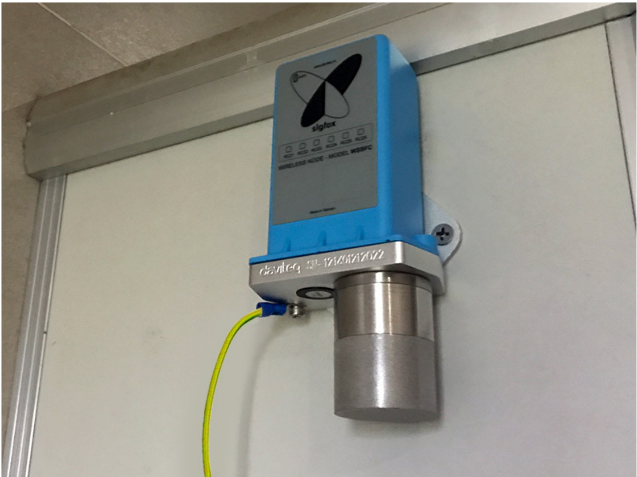
Step 3: Grounding the sensor
