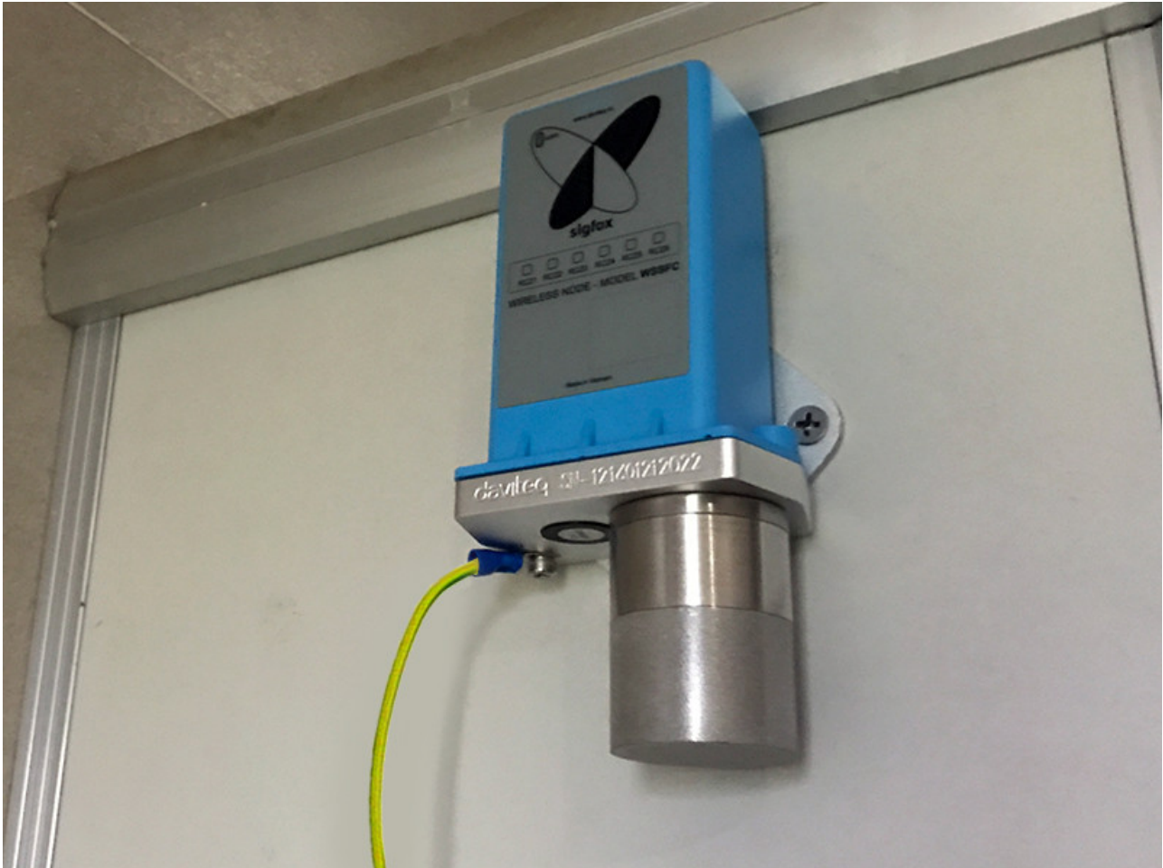
Step 3: Grounding the sensor
