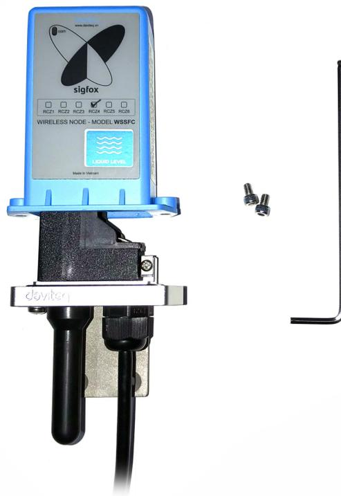
**Step 4:** Plug the connector to the configuration port;
