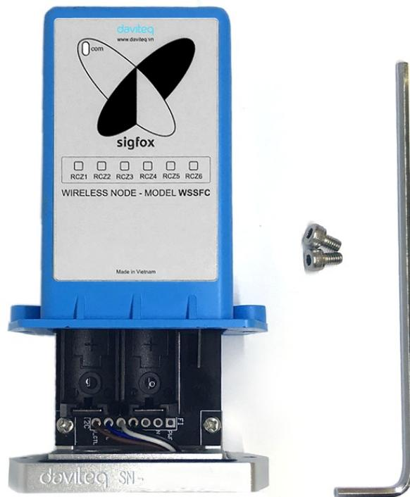
**Step 2:** Insert 02 x AA 1.5VDC battery, please take note the poles of the battery
