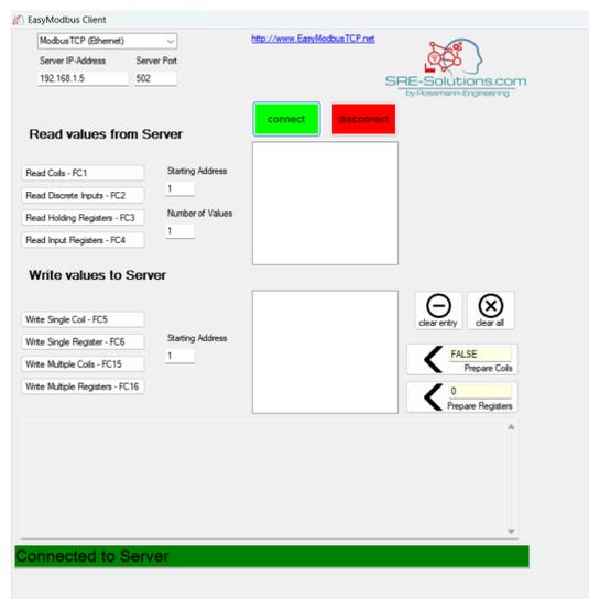
**w** Ensure that the IP address of the PC is configured within the same subnet as the TCP/IP server address set on the iConnector in Step 1.
