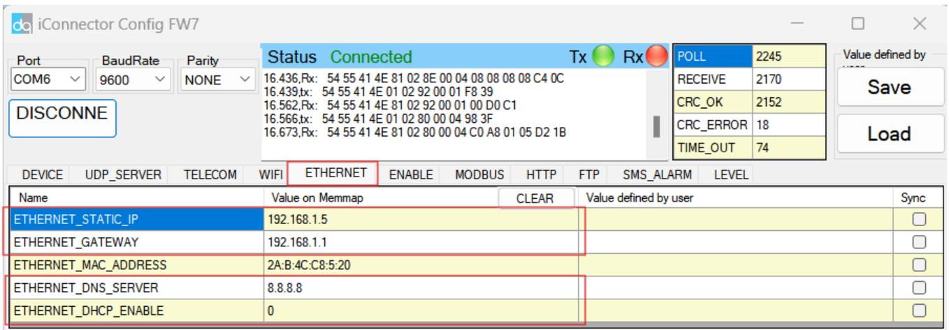
The parameter **MAIN\_NETWORK** is located in the WIFI tab of the software, while other parameters are in the **ETHERNET** tab.
