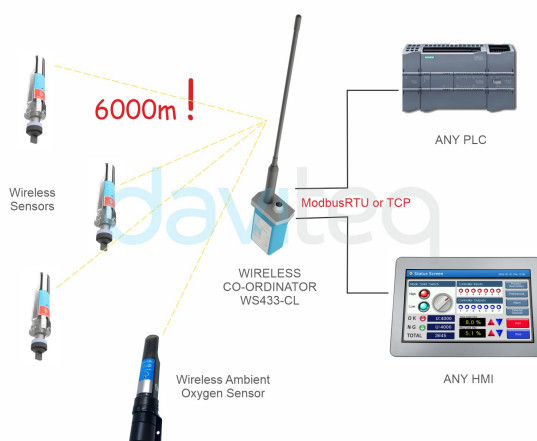
CONNECT WIRELESS SENSORS TO any PLC or HMI
