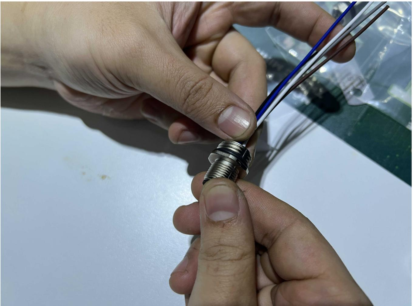
**Step 9:** Re-assemble the 03 inside M12 connectors to housing and lock them tightly with nut.
