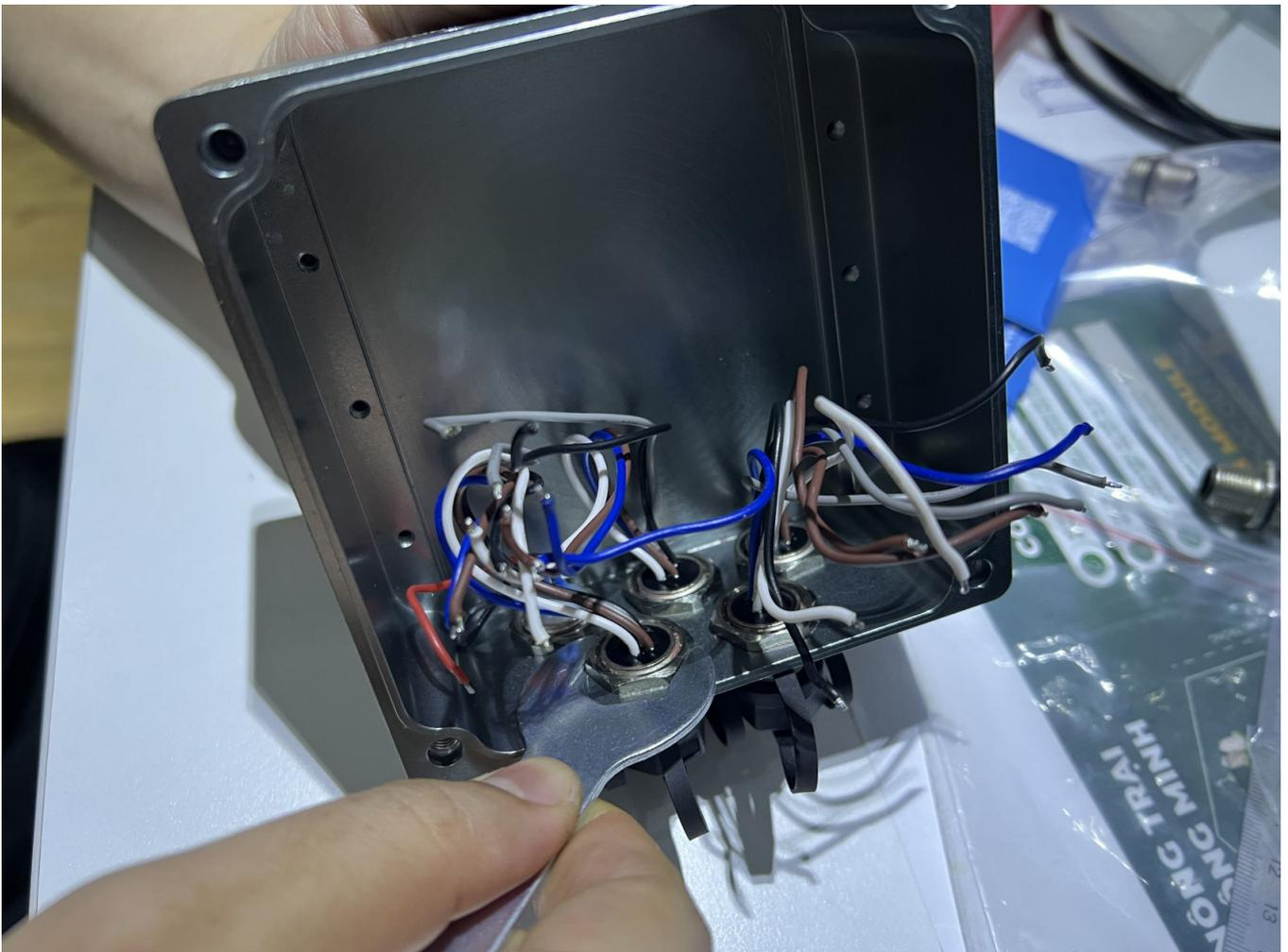
**Step 6:** Move the 02 outside connectors a bit further out, so that you may have more clear space to access the nuts of 3 x M12 connectors inside.
