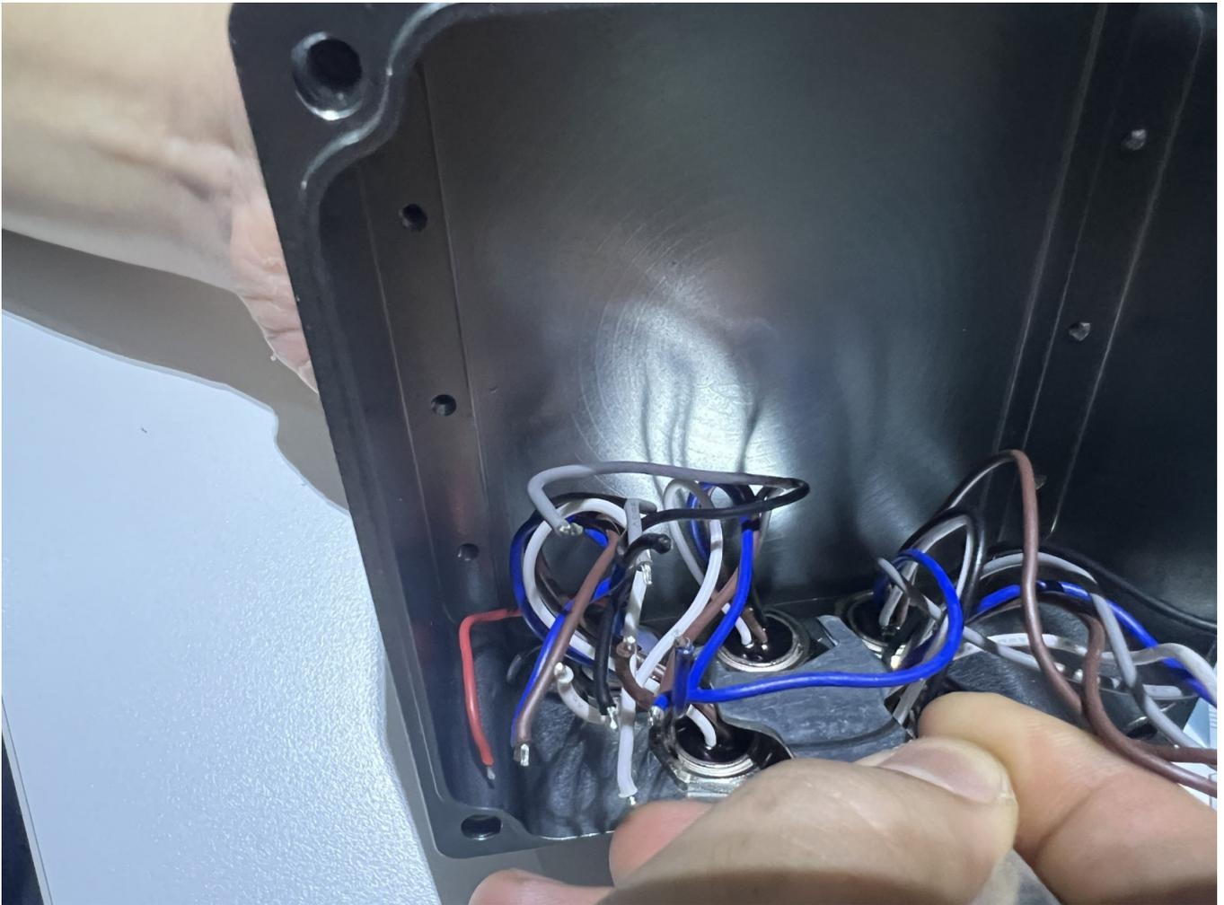
**Step 8:** Remove the thin-gasket (attached with connector cover), and insert the new O-ring from the front side of connector. Repeat this step for 03 inside connectors.
