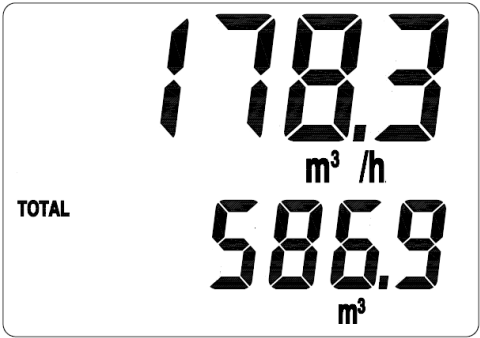
Picture 7.2: Flow rate and total flow
