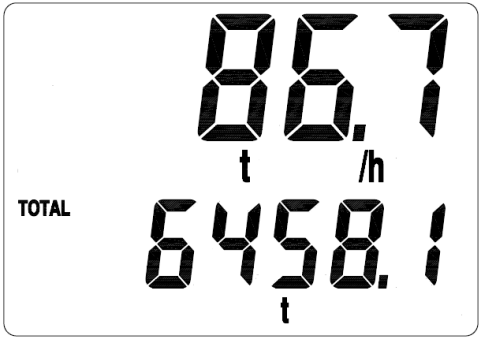
Picture 7.3: Mass flow and total flow of steam displaying
