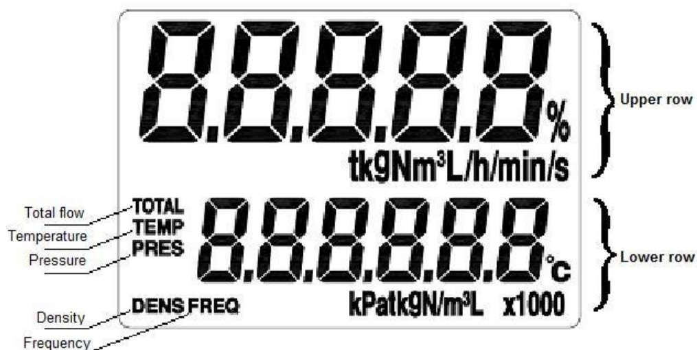
Picture 7.1: LCD display
