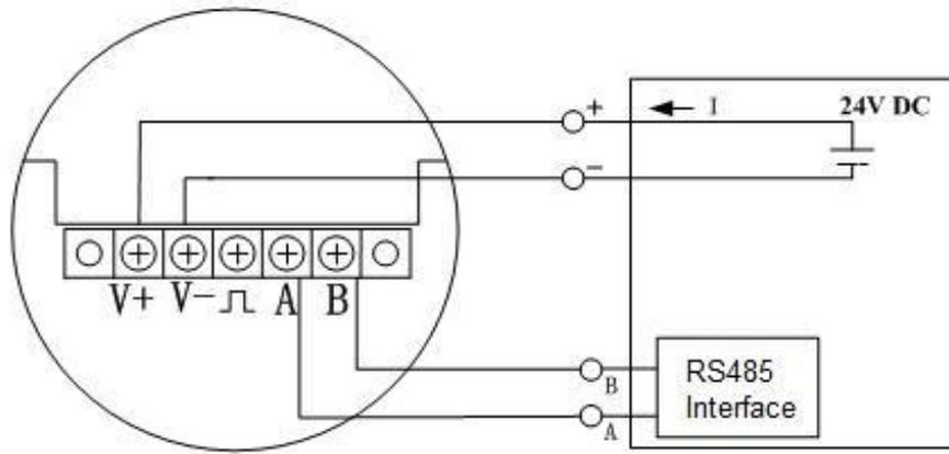
Picture 6.5: Wiring for RS485
