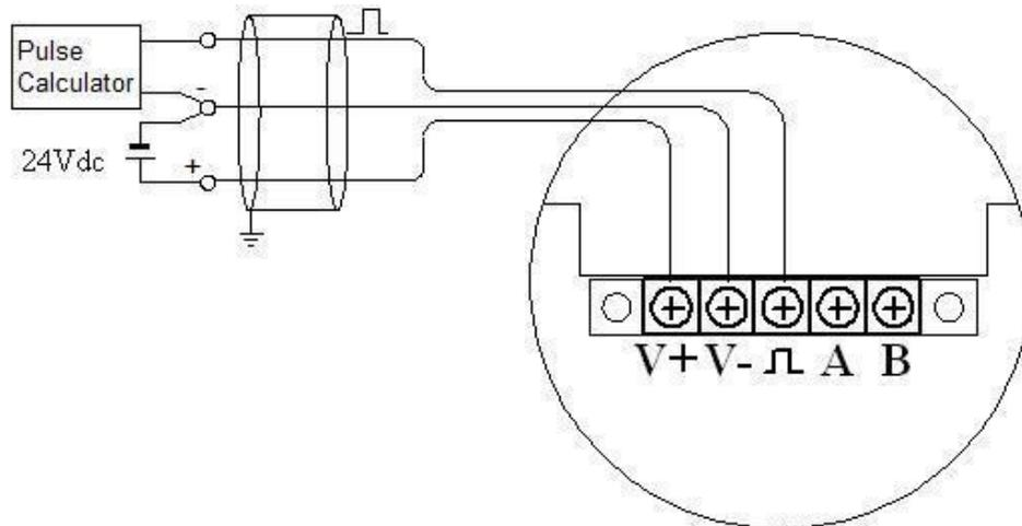
Picture 6.3: 3-wire pulse output wiring
