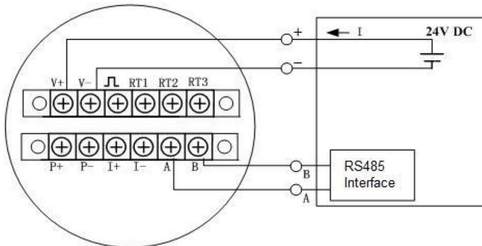
Picture 6.9: Wiring for RS485
