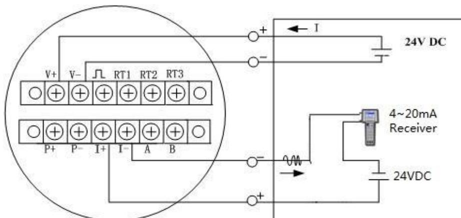
Picture 6.7: Wiring for 4-wire 4~20mA
