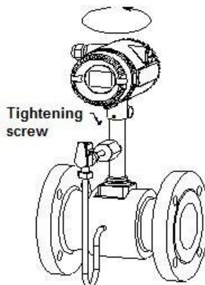
**Picture 11.1:** Reverse the transmitter front and back
