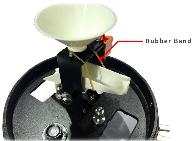
**Step 3:** Fix the sensor pins and adjust the height of the pins so that the bubble inside the sensor is centered.
