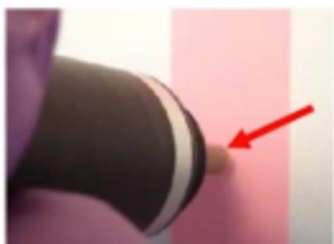
4. Polish the working electrode (WE) surface (see arrow) with the polishing strip until it is shiny in appearance.
