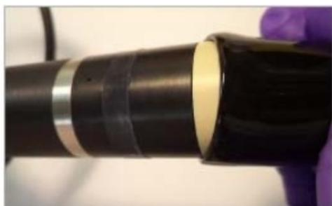
2. Remove the protection boot from the electrode or membrane cap
