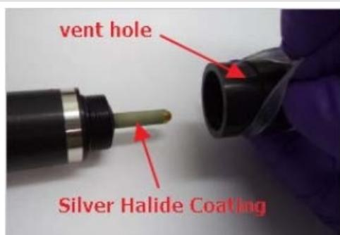
3. Lift the silicone band covering the vent hole. Make sure the vent hole (see arrow in image) is open to air. Avoid using any sharp tools for this step. Set the membrane cap aside.
