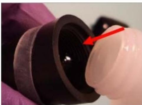
5. Fill the membrane cap with Internal Filled Gel (IFG) to the upper threads (red arrow).
